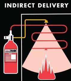
With the Indirect Low Pressure (ILP) System, the Firetrace Detection Tubing is used only as a detection device. The fire suppression agent is delivered via copper tubing, stainless steel tubing or braided hose. Once the tube "bursts", the suppressant is discharged through strategically placed nozzles within the protected enclosure.
