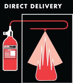
The Direct Low Pressure (DLP) System utilizes the Firetrace Detection Tubing as both the fire detection device and the fire suppressant delivery system. The portion of the tube nearest the hottest point of the fire ruptures, forming an effective discharge "nozzle". The pressure drop in the tube releases the entire contents of the cylinder through this nozzle.
